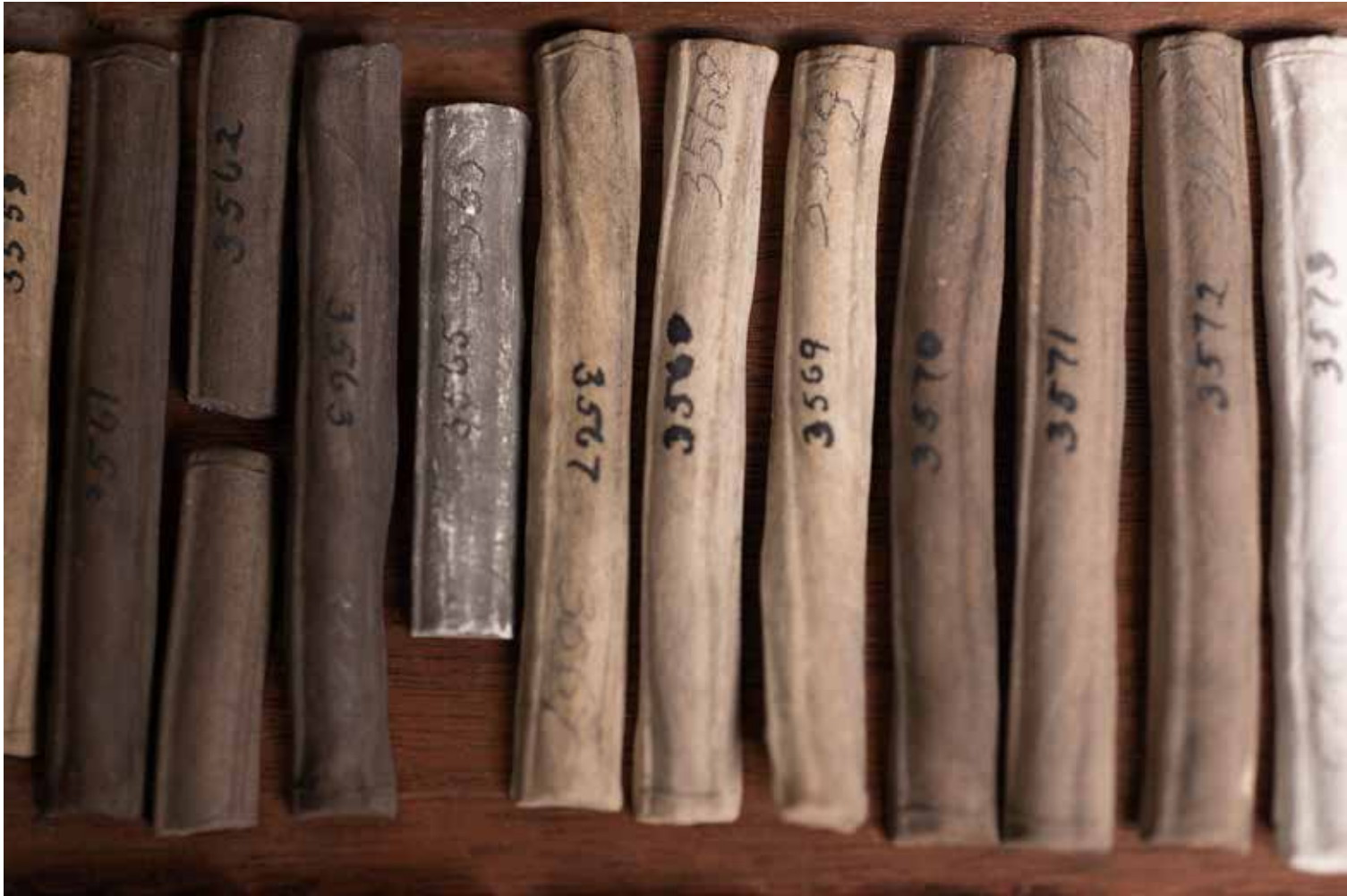
Fig. 10. Detail of a tray with various ceramic trials, made at the factory of Josiah Wedgwood, Etruria, Staffordshire, 1759-1795, museum number WE.7405-2014. Shown are trials for 'various compositions with clay, in order to make a body to diminish in burning as much as possible, upon the idea of forming a thermometer'. Photo © Victoria and Albert Museum, London.
