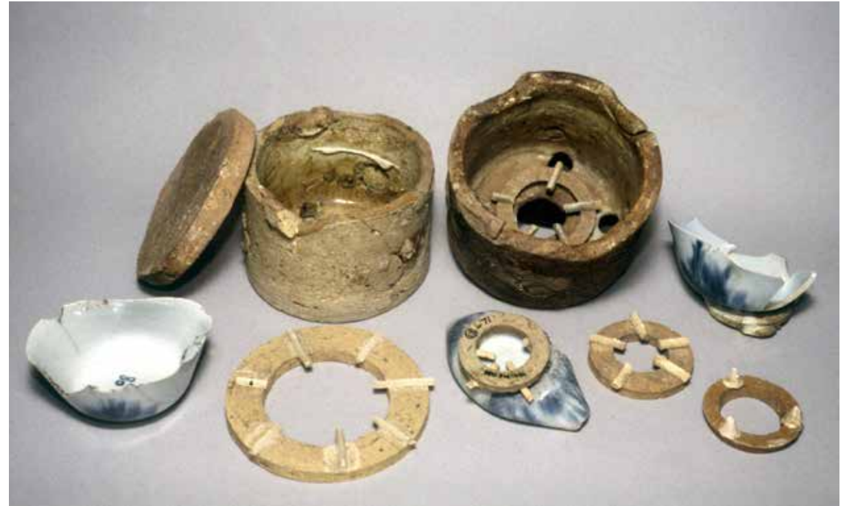
Fig. 19. Saggars, saggur cover, soft-paste porcelain teabowls and the stilts upon which they were fired from the Longton Hall excavations; 1751-1760
