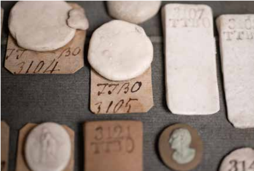
Fig. 3. Detail of a tray with various ceramic trials, made at the factory of Josiah Wedgwood, Etruria, Staffordshire, 1759-1795, museum number WE.7137-2014. Details also showing trial 3107, containing ingredient 23, Cherokee clay. Wedgwood comments: 'A very fine white body, perfect porcelain and seems to stand well.' Photo © Victoria and Albert Museum, London
